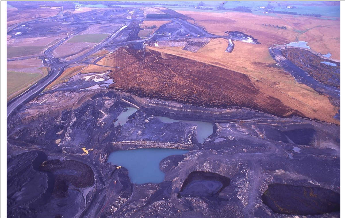
Figure 2. Mining of fire clay from beneath a raised bog in the Central Belt of Scotland. The peat face has collapsed in a series of concentric half-circles, leading to significant impact into the main peat body.
