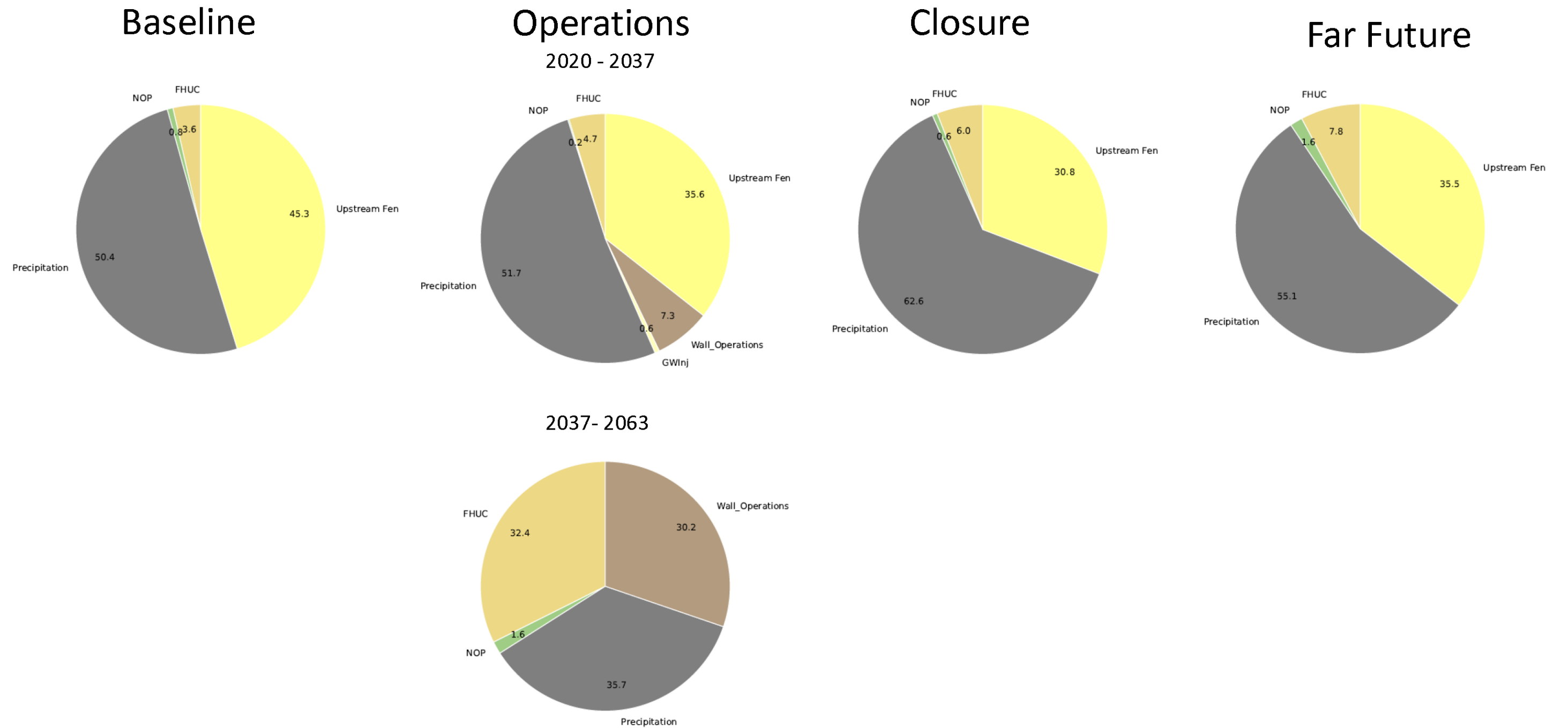
Figure 4.3-17: Predicted Proportions of Water Types in the Non-mined Fen for Historical Climate Scenario: Baseline, Operations, Active Closure, and Far-Future Timeframes
