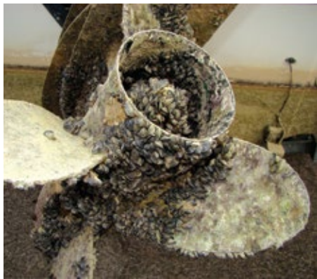
Quagga mussels on boat propeller PHOTO: US NATIONAL PARK SERVICE, LAKE MEAD NATIONAL PARK
