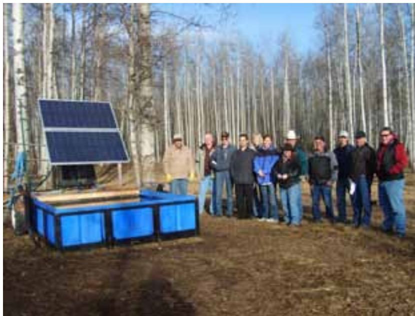
A demonstration off-site livestock watering system managed by Rocky Riparian Group, now Clear Water Landcare. For five years, this solar-powered system was loaned out to help people discover the technology’s potential.
