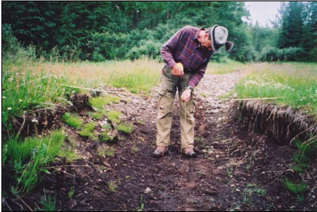
Figure 3. Measuring the depth of an Erosion Event along RNG
