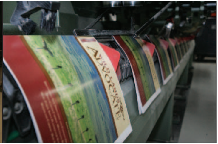
The Advocate on the stitching machine after being folded as a 16-page signature.
