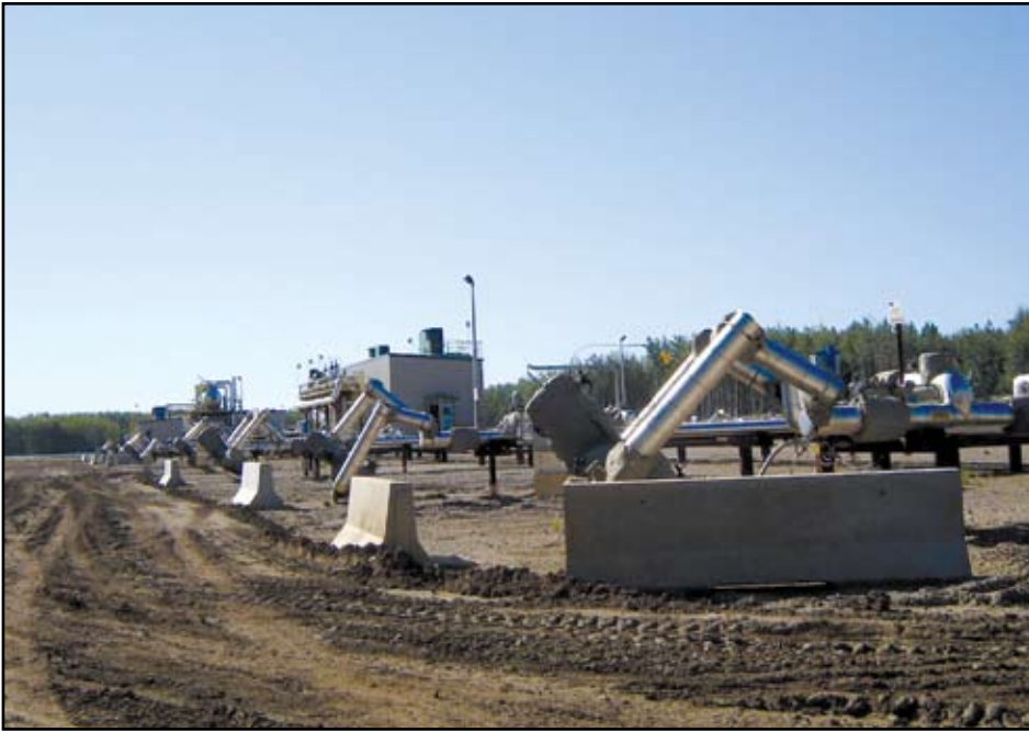
On a Steam Assisted Gravity Drainage (SAGD) project site, a single well pad has many well pairs to steam and pressurize the bitumen so that it may be pumped to the surface.
