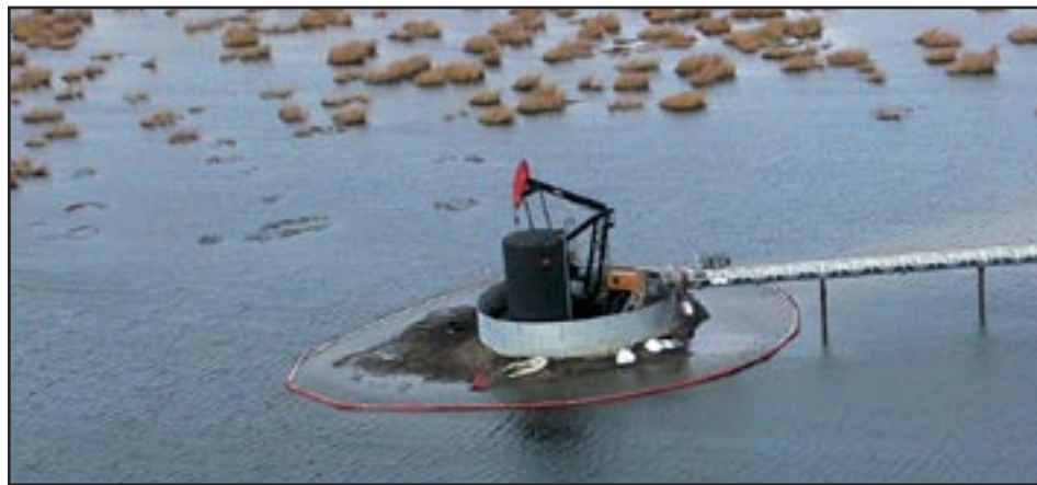
Several small oil spills have occurred in Hay-Zama in the last few years, but the companies involved have contained the spills with booms and mitigated the damage. With oil and gas activity phasing out of the area, the risk of a major spill will gradually diminish until 2017, when industry will no longer be active in the Wildland Park.
